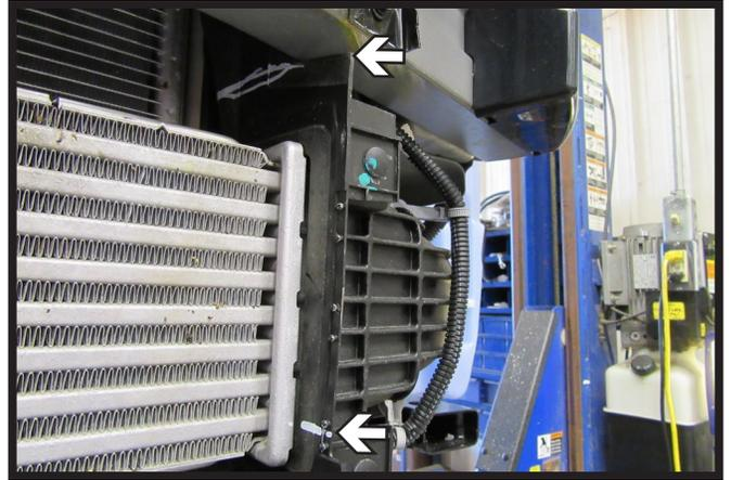
11. Trim the plastic shielding off flush under the bumper and across the bottom as shown. Do this on both sides of the vehicle,
