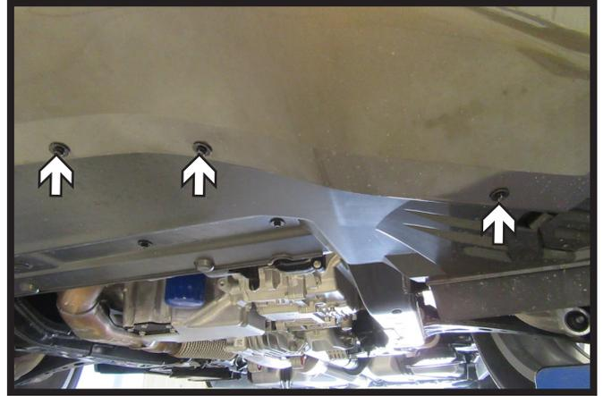
5. Using a 7MM socket, remove the ten (10) bolts from the underside of the fascia. There are five (5) on each side.
