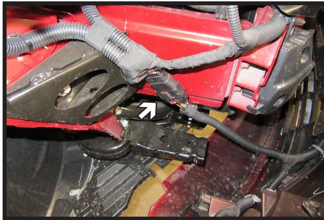
6. Pull the corners of the fascia away from the vehicle. Then unplug the electrical harness on the passenger side of the vehicle. Remove fascia and set aside to be reinstalled later.
