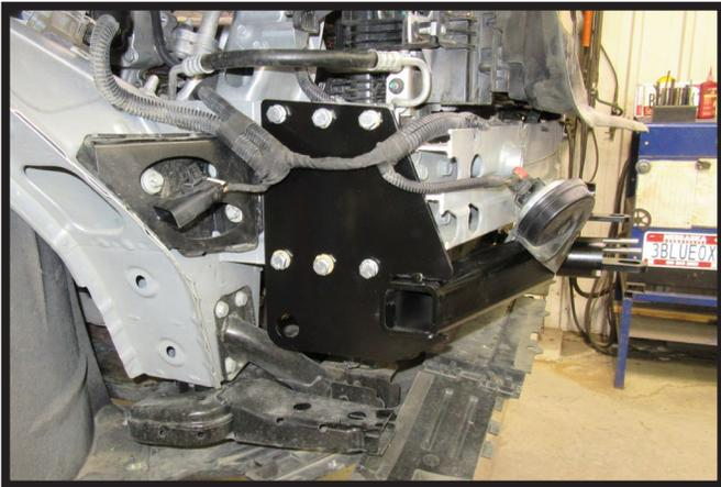
15. Install baseplate so that it is flush with the top and front lips of the frame. Level and clamp into position.
