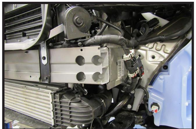
13. Using a reciprocating saw, trim the end of the bumper flush with the outside of the frame. Do this on both sides of the vehicle.
