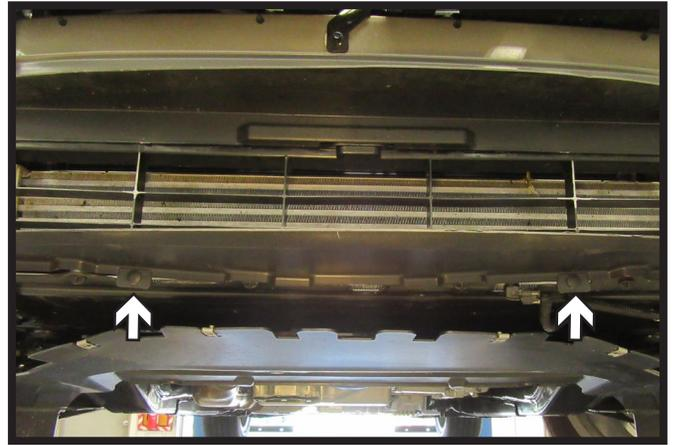
7. Remove the eight (8) push pins from plastic housing. There are four (4) on the top, one (1) on each side and two (2) on the bottom. Remove plastic housing and set aside, it will not be reinstalled later.
