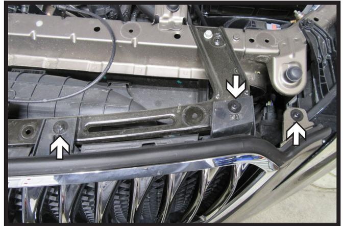
2. Using a T15 Torx, remove the six (6) bolts from the top edge of the fascia. There are three (3) on each side.
