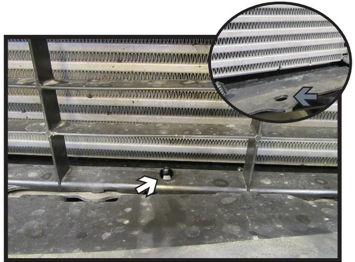
9. Remove the temperature sensor and let hang it will be relocated later.
