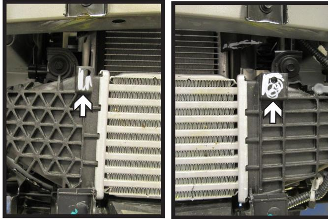
14. If needed use a reciprocating saw to trim the indicated areas on both sides of the vehicle so that they are flush with the frame.
