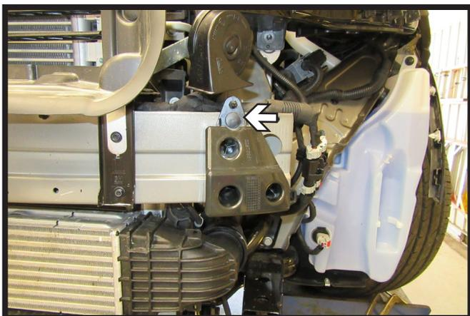
12. Remove the push pin from plastic reinforcement on the bumper face and set aside, it will not be reinstalled later. Do this on both sides of the vehicle.
