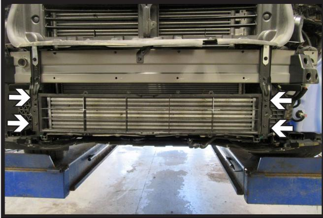
8. Using a T25 Torx socket, remove the four (4) bolts from the lower grille and set it aside. It will not be reinstalled.
