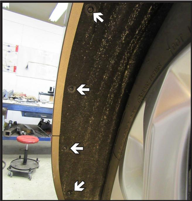
3. Using a T15 Torx socket, remove the four (4) bolts from the wheel well liner. Do this on both sides of the vehicle.
