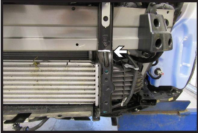
10. Using a reciprocating saw, trim the bracket flush with the bottom side of the bumper. Do this on both sides of the vehicle.
