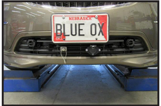
18. Hold the fascia as close to its original position, mark and trim the fascia around the convenience links and attachment tabs. Reinstall the fascia, fascia cover, and reconnect all electrical connections.
