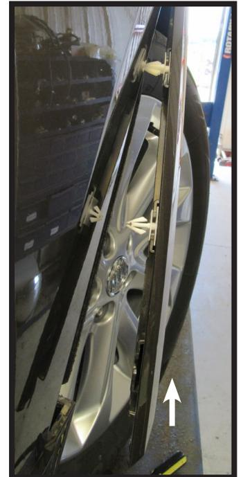
4. Pull back the wheel well liner. Using a 7MM socket remove the bolt (gray arrow). Then release the clips from the fender flare (left, white arrow). Pull straight up on the flare to release the bottom and then out away from the vehicle. Do this on both sides of the vehicle.
