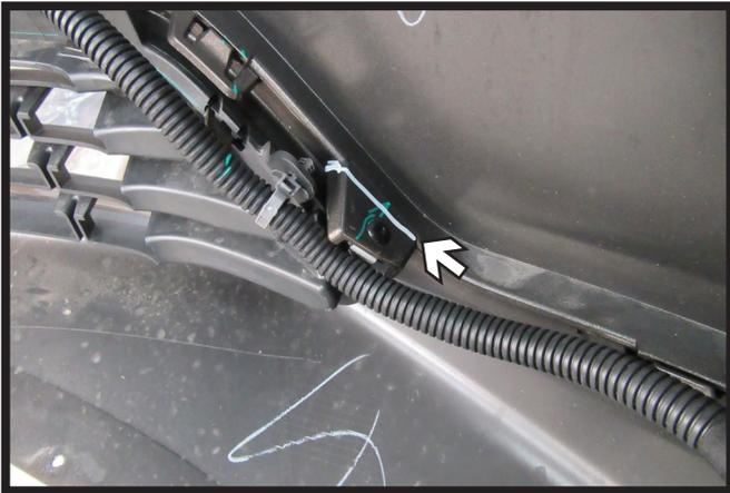
17. On the backside of the fascia, trim the lower tab back flush with the lip. Do this on both sides of the fascia.
